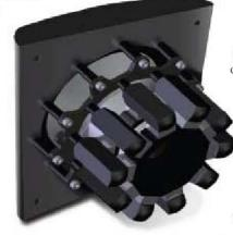
Neodymium rod magnets separated from the chassis by soft-iron sections and placed in front of and behind the voice coil in a patented, push/pull arrangement. The rear of the driver is left completely open and this means that there is no reflection back into the cone and far less mechanical or thermal compression. The whole driver has been stripped back to the bare essentials, the cage replaced by stand-offs in the effort to further eliminate reflective surfaces.
